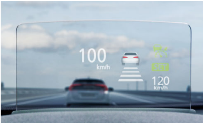
The color Head Up Display unit makes driving safer by presenting vehicle speed, data from the active safety systems and other necessary information that minimizes eye movement and provides instant readability.
